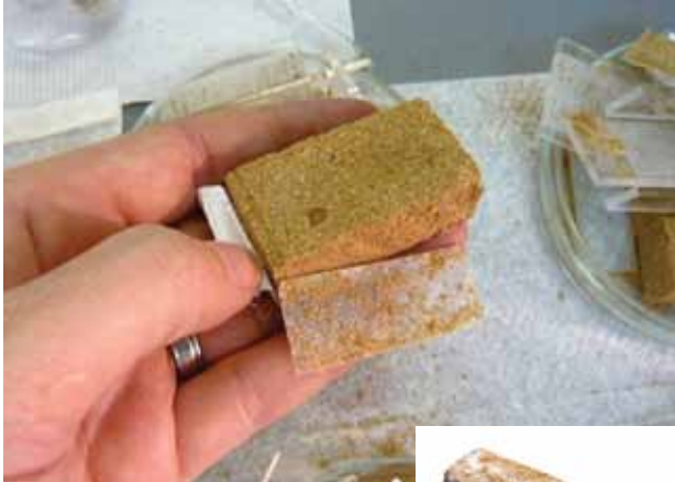
Ginger Krieg Dosier created a biomanufactured brick that can be manufactured on site with a 12-step process involving placing a formwork in sand, adding bacteria, cementing solutions and time.
